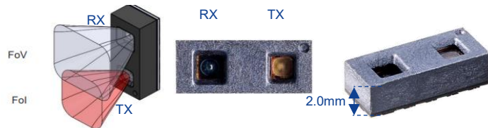
Multi-zone 3D-dToF sensors (~proximity sensors)
