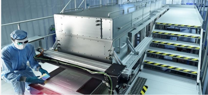
Solid-State Laser Lift-Off (LLO) System
